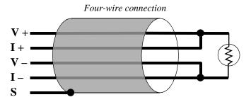
Like the three-wire circuit, separate conductors are run from the V- and I- terminals to the sensor. In addition, separate conductors are run from V+ and I+ to the sensor, where they are tied together. This circuit eliminates cable loss effects from both the V+ and V- lines.
