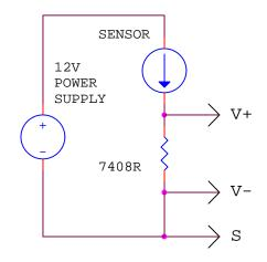
If the external power source is not isolated (i.e., its negative output terminal is connected to the backplane power supply return), you should not connect to the S terminal as shown in the above diagram, as a potential ground loop would be created. In such a case, leave the S terminal disconnected and connect to the V+ and Vterminals only.
