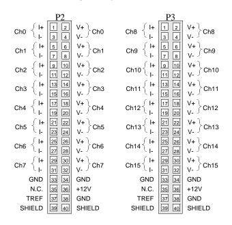
Sensor channels 0 through 7 connect to header P2.
