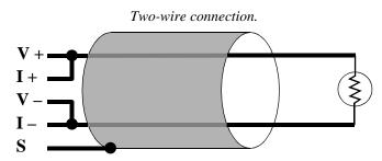
This circuit conserves wire, but it causes measurement error due to the voltage drop between the TB and sensor. There are two potential solutions for this problem: use short wires, or use more than two wires.
