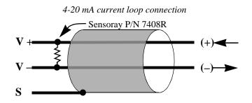
It is important to note the Smart A/D does not provide excitation for current loops. Current loops must be energized from an external power source, such as the isolated 12V power supply in the following schematic:
