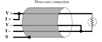
In this situation, the high impedance V- terminal detects the voltage at the sensor before any voltage drop can occur.
