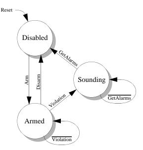
Initially, all channel alarms are disabled and each channel is in the Disabled state. The SetAlarmEnable function is used to switch between the Disabled and Armed states.
