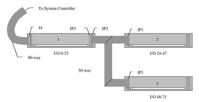
Figure 4 Multiple board configuration
