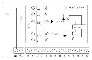
Figure 3 Schematic representation of DC output module in the first I/O position on the board.
