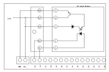
Figure 2 Schematic representation of DC input module in the first I/O position on the board.
