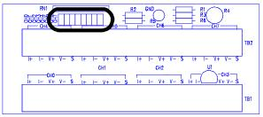
Some Smart A/D<sup>TM</sup> products have built-in OSD option shunts. Do not install any OSD option shunts on the TB if your Smart A/D<sup>TM</sup> has built-in OSD option shunts; instead, install OSD shunts only on the Smart A/D<sup>TM</sup>. As for which channels should have OSD enabled, refer to your Smart A/D<sup>TM</sup> instruction manual for the recommended practice.
