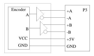
Many encoders utilize single-ended TTL or CMOS compatible outputs. If you are using this type of encoder, connect the encoder A output to the +A input and connect the encoder B output to the +B input. Leave the -A and -B inputs disconnected:
