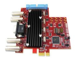
uncompromising capturing of multi-channel video/audio sources in a PCI Express form factor, such as broadcast-grade video/audio capturing, video surveillance, law enforcement, and traffic monitoring.
