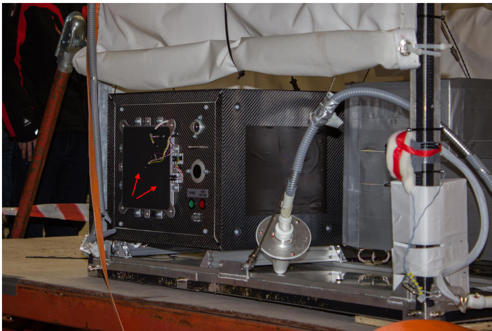
Figure 4.5: POLARIS on the BEXUS 18 gondola after recovery. The two red arrows highlight the only visible damage which are some light scratches on the coating of the external plate
