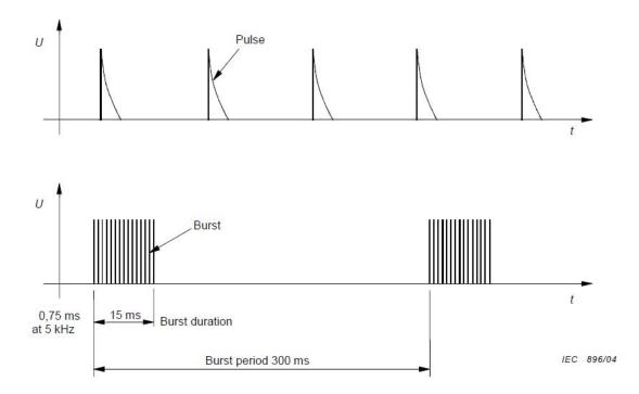
The waveform of the transient can be seen in the following figure.
