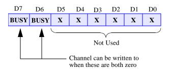
The status register contains two **BUSY** bits that are used to handshake data onto the Model 7405 board. When both bits are reset to logic 0, the board is ready to accept new data. The remaining six bits are not used and should be ignored.
