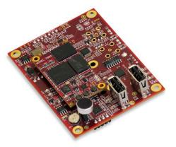
The board encodes standard NTSC/PAL composite video using efficient
