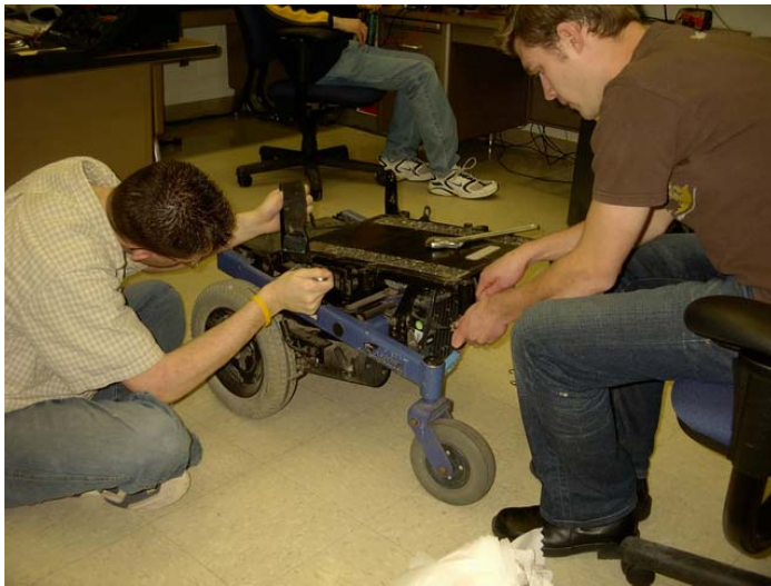
Figure 3: Stripping the chassis of unnecessary parts
