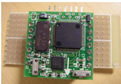
Figure 4: PNI V2Xe compass in place on the carrier board.
