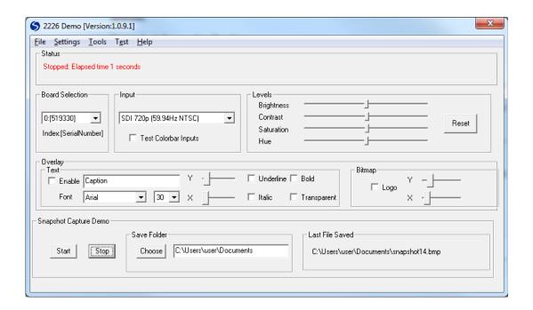
To use the snapshot, first connect and power on your camera source to the 2226. In the demo, select the corresponding input. The next step is optional. If desired, you may change the target output directory. Once this is done, you may click "Start" and snapshots will be captured.
