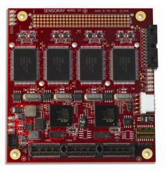
A 24-pin header provides convenient access to all I/O signals on the board. The board's PCI/104-Express connectors support both stack-up and stack-down, and its full conformance to the PCI/104-Express specification guarantees that it won't mechanically interfere with adjacent boards.
