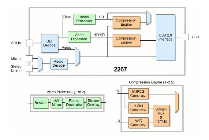
Fig.1. Model 2267 block diagram.
