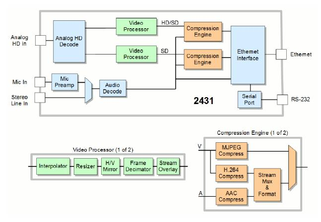
The video processor implements efficient H.264 video compression, producing output data formatted as either MPEG transport stream (MPEG-TS) or in MP4 or AVI file formats. Audio compression is performed using AAC-LC. The stream multiplexer employs high precision hardware timestamps to ensure perfect audio-video sync on players. Snapshot capture is also supported, with MJPEG compression available for both snapshots and AVI streams.
