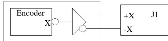
For a single-ended TTL or CMOS index, connect to the -X pin and leave the +X pin disconnected:
