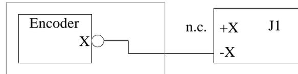
Leave both +X and -X disconnected if you are not using the index input.
