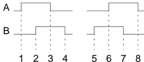
Valid transitions depend on the operating mode. The table to the right lists valid transitions for each mode. In mode 0, for example, a counter will count up only at transitions 6 and 8, and will count down only at transitions 1 and 3.
