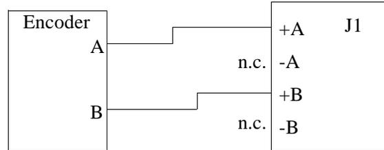
Counter channels may also be interfaced to single-phase devices. In such cases, the counter mode is set to 3 or 7, and the device is connected as follows:
