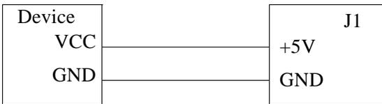
If you are supplying power from an external source, make sure the device ground is connected to one of the GND pins on J1:
