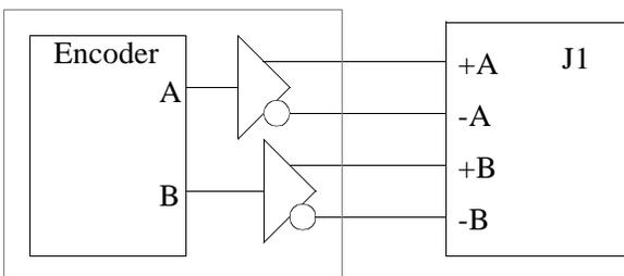
Other encoders have TTL or CMOS outputs. If you are using this type of encoder, connect it as follows:
