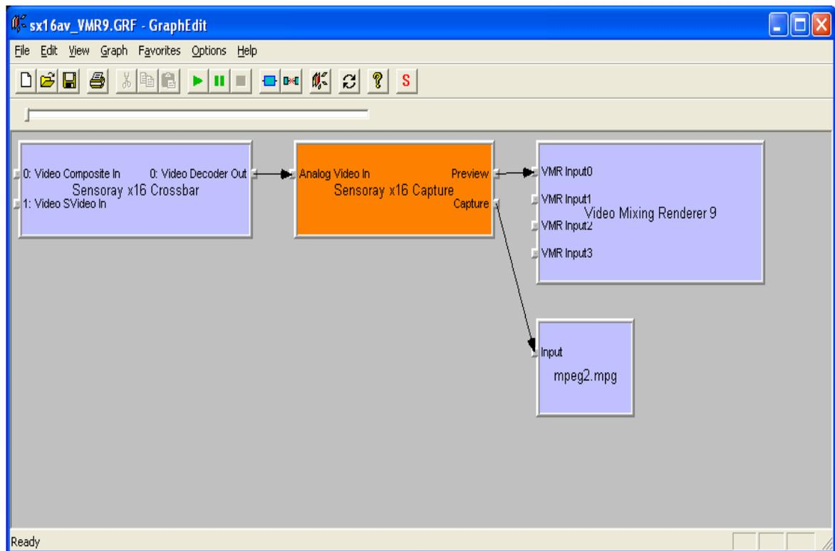
The crossbar allows selection of S-Video/Composite inputs on the 616.
