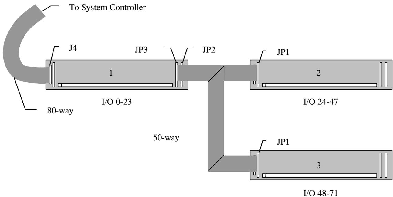
Figure 4 Multiple board configuration
