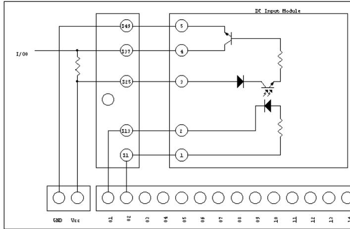
Figure 2 Schematic representation of DC input module in the first I/O position on the board.
