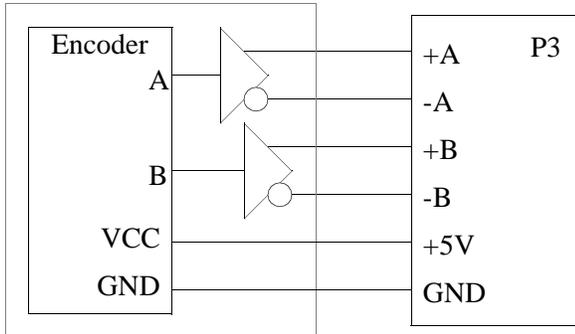
Many encoders utilize single-ended TTL or CMOS compatible outputs. If you are using this type of encoder, connect the encoder A output to the +A input and connect the encoder B output to the +B input. Leave the -A and -B inputs disconnected:
